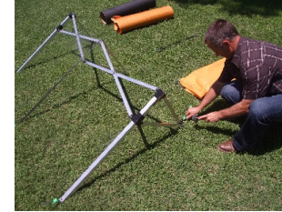
Stake the two back struts
